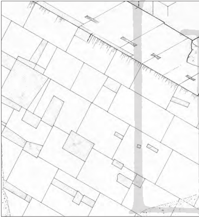
Fig. 1 Pyramid of Senwosret I. Patch stones covering the casing of the west side. (D. ARNOLD, The Pyramid of Senwosret I , in: MMA Egyptian Expedition 22 , New York 1988, Pl. 93a, Drawing D. ARNOLD)
